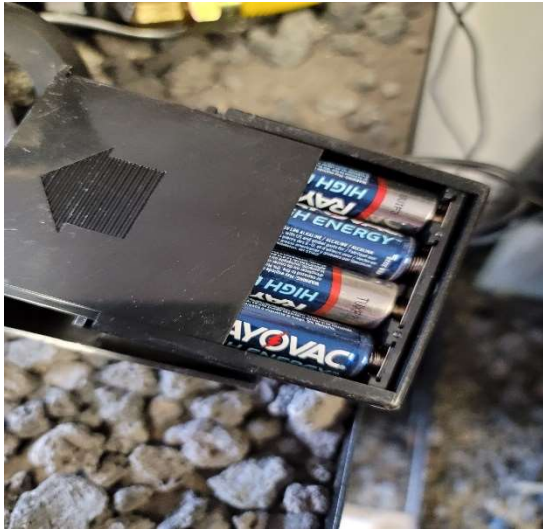
Figure 5 – Underside of remote receiver box where batteries are installed. Cover just slides off
