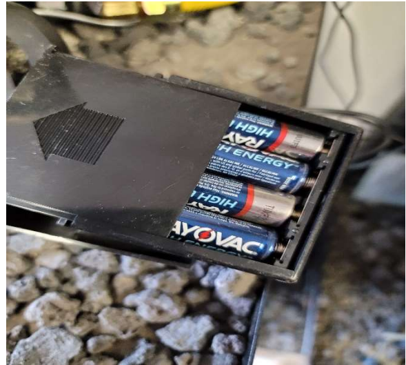
Figure 6 – Underside of remote receiver where batteries go – cover just slides off
