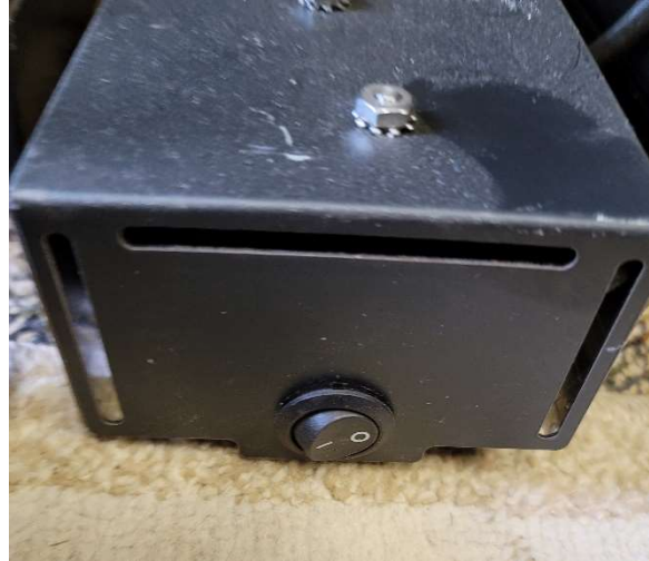
Figure 2 – Larger ignition box. Takes 2 D batteries Older units may have the small box inside this box as well. Older units will not have a toggle switch on the front as pictured – just the switch on the smaller box. A Phillips screwdriver is needed to replace the batteries.
