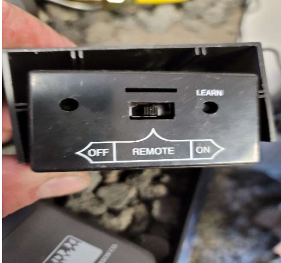
Figure 1 – Remote receiver box. Takes 4 AA batteries.
