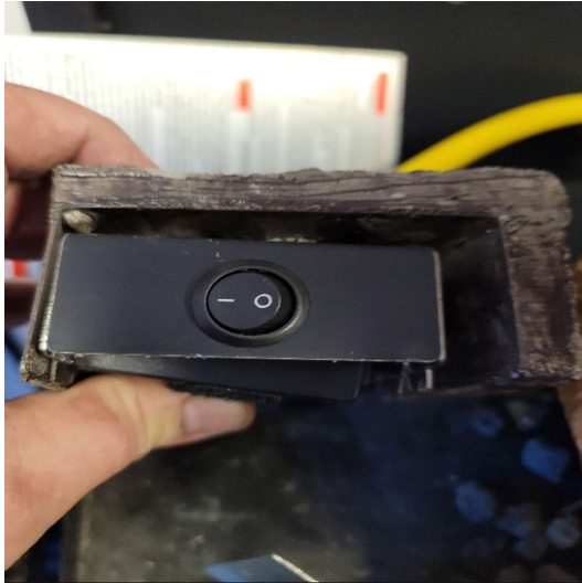
Figure 3 – Battery box on a G31 or G52 unit Takes 4 AA batteries. A very small Phillips screwdriver is needed to remove battery cover.
